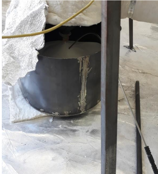
Figure 9. Bulk temperature inspection in the alumina deposit, after the alumina flow ended in the experiment.
